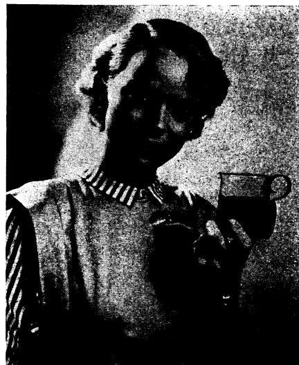
DIRECT SOLDER—The handle of this glass beaker is a metal spoon, soldered to the glass by a process that permits direct joining. Miss Jane Barstow of the General Electric Company is holding the "cup."
