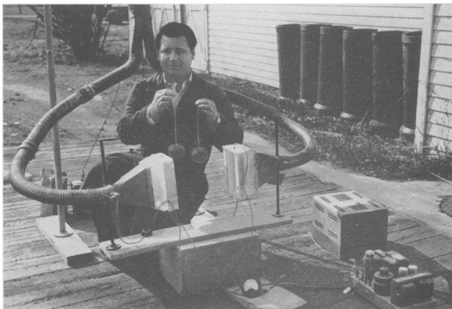
ELECTROSTATIC DUSTING —Henry D. Bowen, Michigan State College graduate assistant, who developed the electrostatic dusting process, shows here how the method works. The apple on the left became coated when held in the charged dust, while the one on the right, although receiving the same amount of uncharged dust, remained uncoated.
