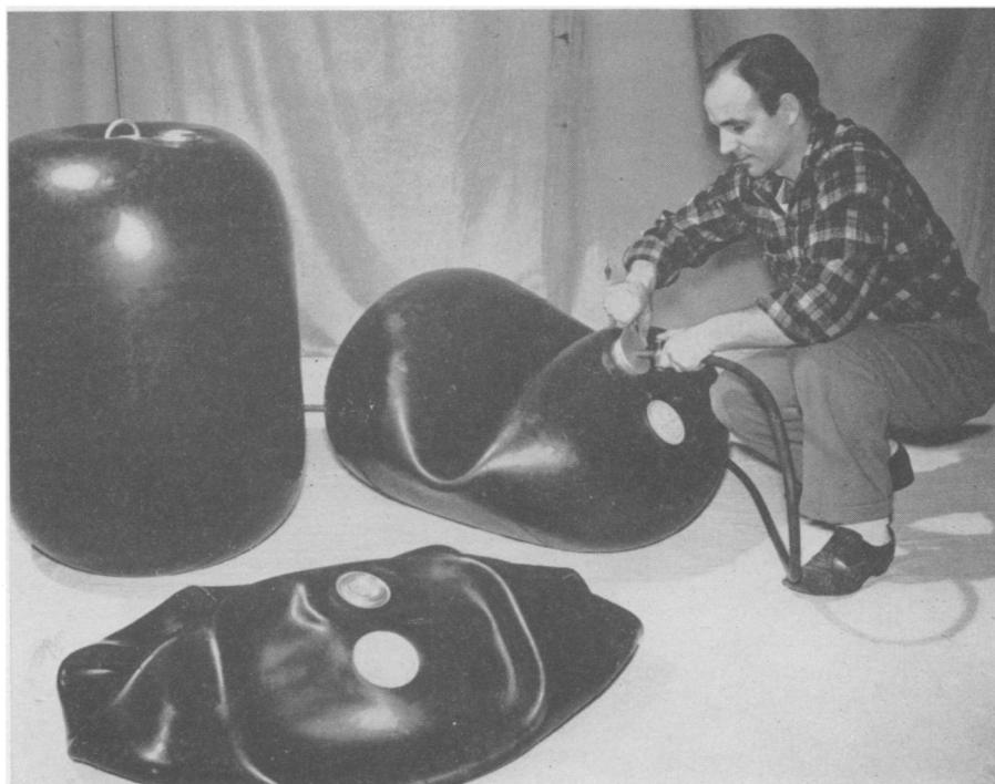
RUBBER SHIPPING DRUM —The new 55-gallon rubber drum suitable for shipping liquids is shown in three stages. At left is a filled drum, in the foreground, a collapsed drum, and at the right a drum being filled, for which no vent is needed. Since the drums collapse when empty, valuable shipping space can be saved when they are being returned.
