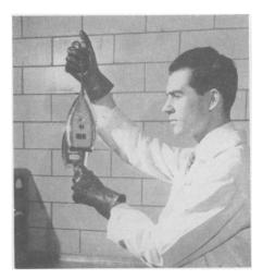
ELECTROPLATED METAL—The gleaming finish on this electric iron cover shows the metal plating technique developed by engineers of Westinghouse Electric Corporation. The new method is expected to save huge quantities of nickel, a strategic metal.
