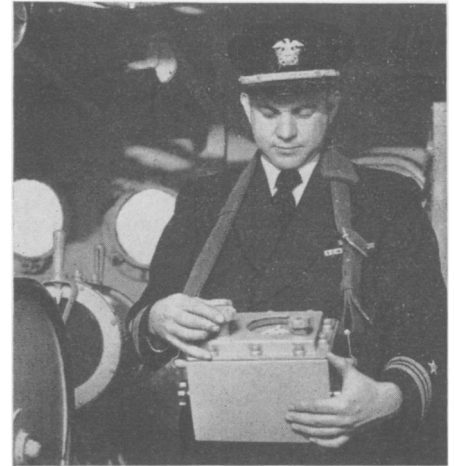
ELECTRIC HELMSMAN — Lieut. Comdr. W. M. M. Fowden, Jr., demonstrates one of the units by which ships can be steered from widely-separated positions on board.
