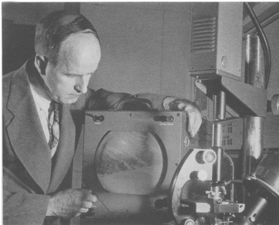
TELEVISION STARS — Wiggling microscopic insects and slides of animal tissue are the star performers on this set, a television microscope designed by RCA Laboratories, being adjusted by Leslie Flory. (See SNL Jan. 20.)
