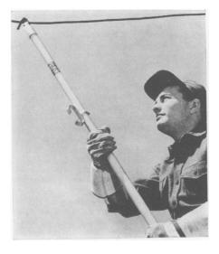
ing high voltage electricity, come in lengths from two to 20 feet and are fitted for the easy attachment of the tools. Many types of tools can be used with this non-conductive pole shown in the picture.
