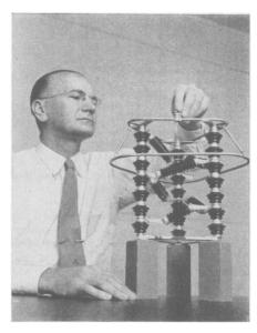
SPIRAL STAIR FOR LIGHT-NING—Model of a new type lightning arrester, developed by Westinghouse Electric Corporation, which sends a stroke in a spiral down the insulated conductors which angle between the vertical columns. The full size arrester is only half as tall as those formerly used and does not require large structural steel supports. BACTERIOLOGY
