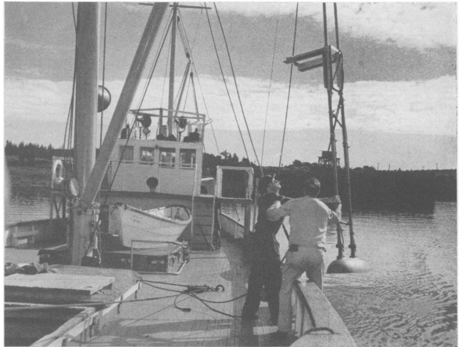
BEDROCK SURVEY —Going over the side to start a day's work is the transmitter of a standard Blutworth depthfinder, used as a check in shallow waters of the more powerful apparatus with which the Bay of Fundy was recently surveyed. The scene is aboard the David C. MacNichol , a coastal freighter pressed into service as a research vessel.
