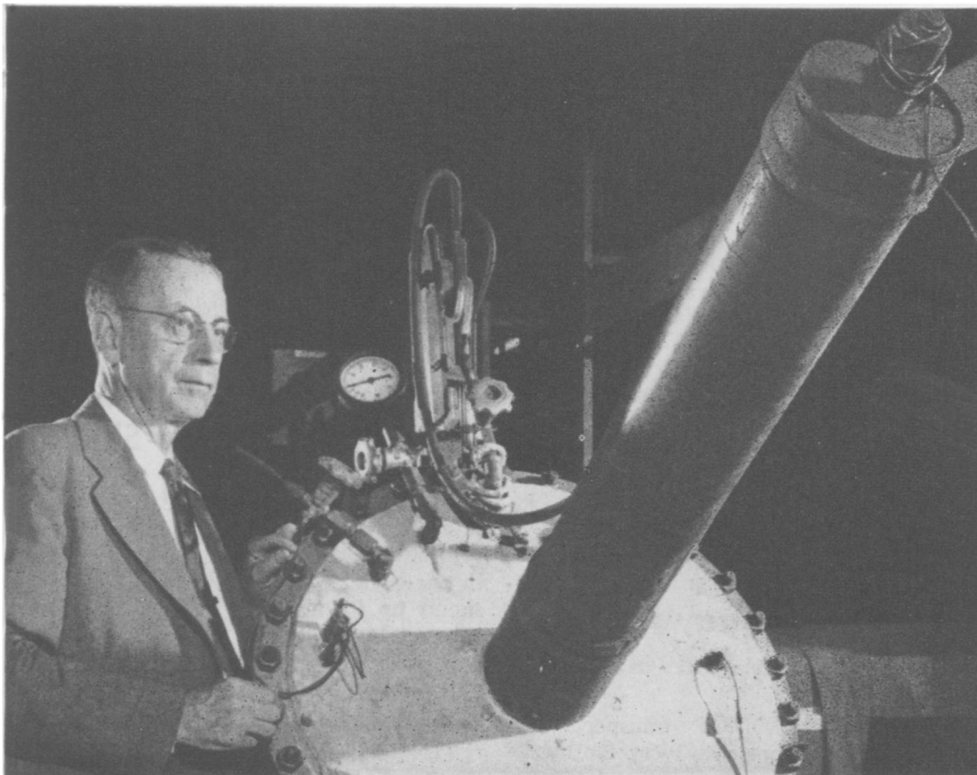
ELECTRICAL "HOWITZER" —Dr. C. F. Hill of Westinghouse Research Laboratories here shows the equipment used to bombard fluorocarbons with electrical strokes ranging up to 300,000 volts to develop cooling spray for transformers.
