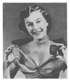
EXPOSURE METER, match-box size and designed particularly for use in taking colored pictures, is shown in the picture. The device is merely pointed at the subject or scene and gives the correct camera setting directly from a scale on its face. No conversions, calculations or special readings are required.
