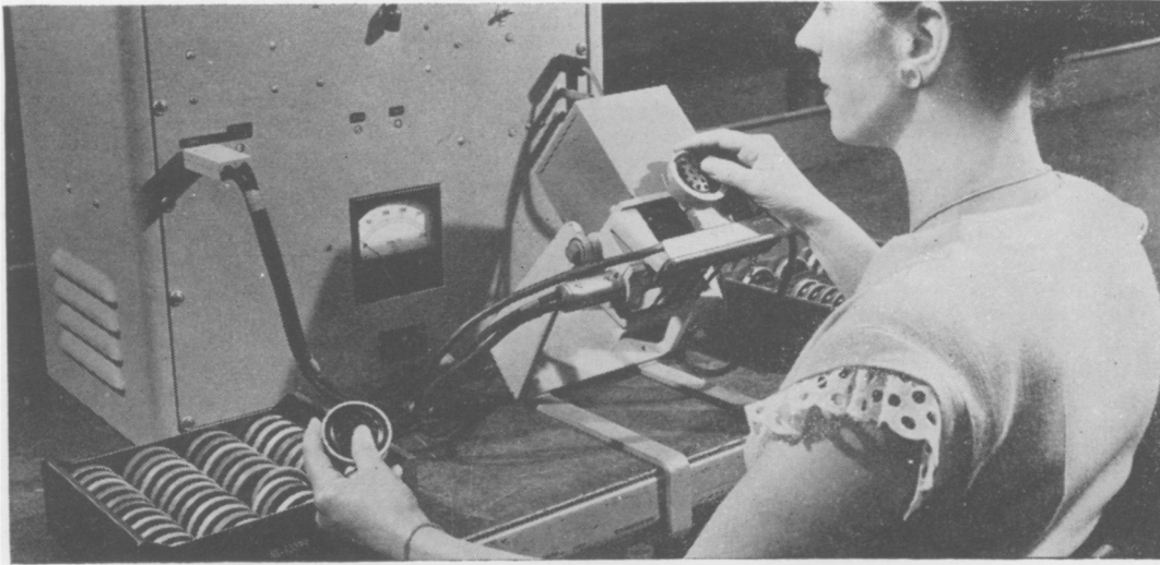
This Western Electric employee mounts a transmitter in the test fixture which is swung down to face an artificial mouth at 45-degree angle, just as transmitters are held in use. More than a million transmitters are tested each year.
