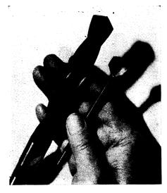
SUPER-FAST DRILL, shown in the photograph, for boring holes in plastics has a straight, round shaft of smaller size than the spiral-grooved shaft found in conventional drills, thus reducing heat from friction. Two tiny notches in the drill tip
