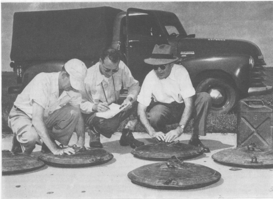
DROPPING LIQUIDS —Before loading for test drops, three engineers check the experimental 5-gallon synthetic rubber containers planned for aerial supply of varied liquids. At right can be seen a standard container.
