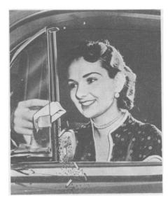
DUMPABLE ASH tray, for use in an automobile, is held inside a hinged vent window, pivoted to a metal clasp that grips the vertical edge of the glass. To empty the tray while driving, one merely opens the vent window and tilts the tray outward
