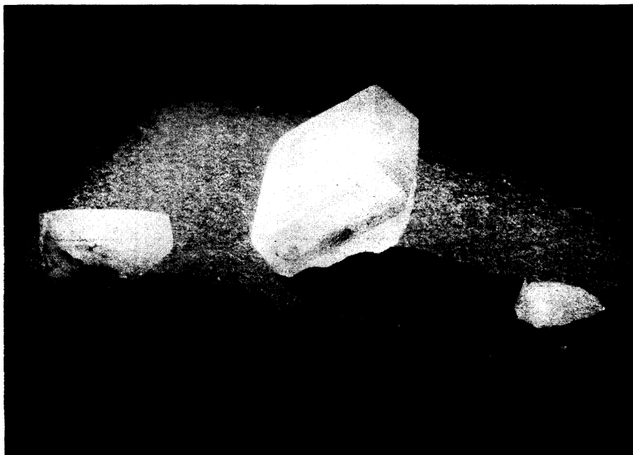
CRYSTAL TRAP —Enlarged clathrate crystals, containing argon trapped in a quinol lattice, have the form shown in this photograph. The actual length of the center crystal is approximately one-quarter of an inch.
