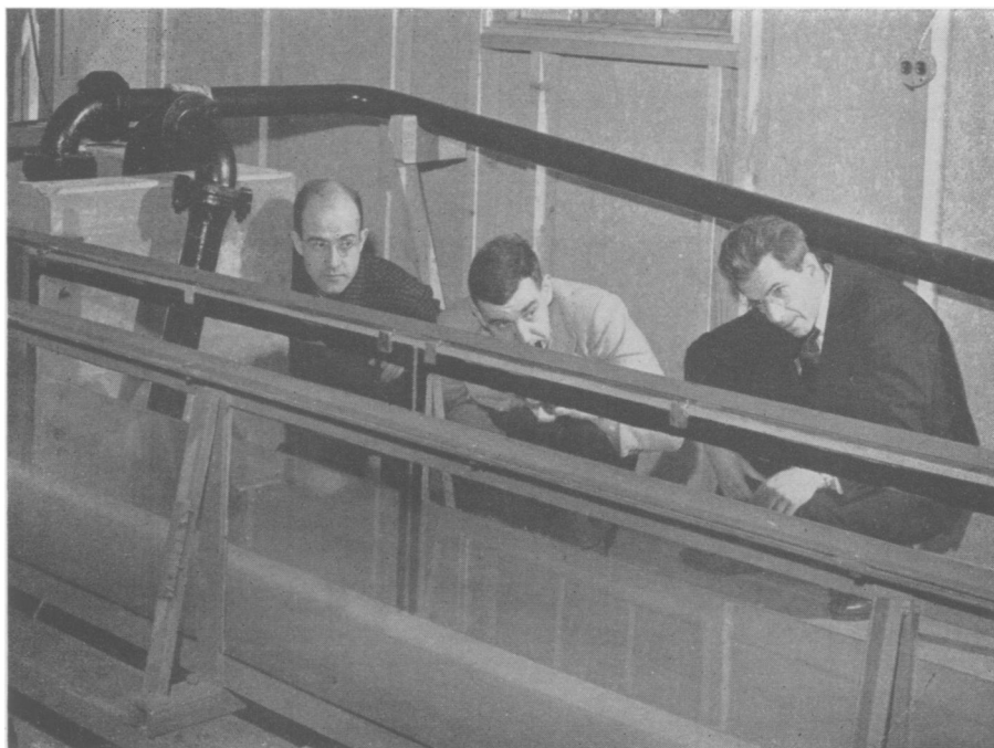
A-BOMB SAFETY FOR HARBORS —Tests in this artificial harbor are helping to tell civil defense experts how much time is needed after A-bomb explosions before entry is safe. Careful scrutiny will show the layer of fresh water on top of salt water in this tidal flushing flume.
