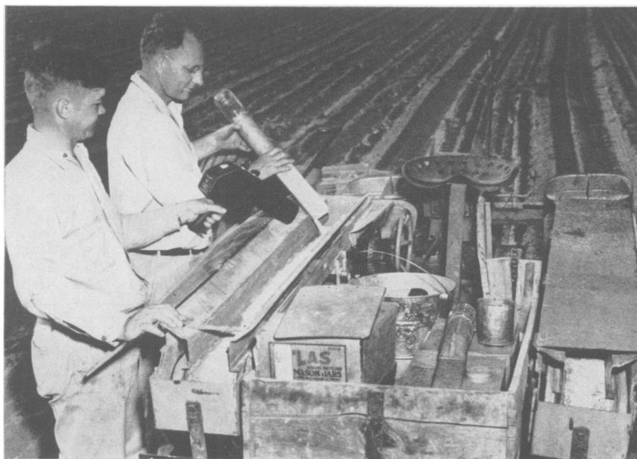
FERTILIZER USE —The best way to place fertilizer is being learned through studies such as this, where radioactively tagged fertilizer, loaded on an endless belt of hoppers, is distributed to a field. One scientist is checking the radioactivity hazard as the "hot" material is poured out through the metal tube.
