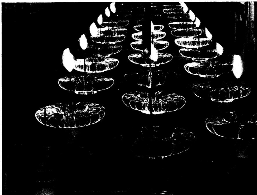
KILOWATT CHINA —Undergoing trial by lightning to reveal any flaws are these ceramic insulators. The white streamers cascading over the porcelain are arcs of man-made lightning, 90,000 volts strong. Electricity jumps from the three solid brass conductor rods to the vertical electrodes placed in the center of each insulator, then flashes over the insulators themselves.
