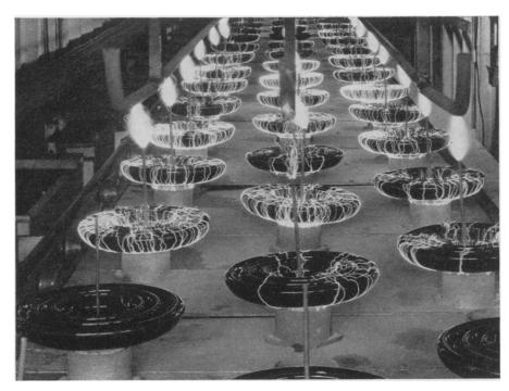
KILOWATT CHINA—Undergoing trial by lightning to reveal any flaws are these ceramic insulators. The white streamers cascading over the porcelain are arcs of man-made lightning, 90,000 volts strong. Electricity jumps from the three solid brass conductor rods to the vertical electrodes placed in the center of each insulator, then flashes over the insulators themselves.
