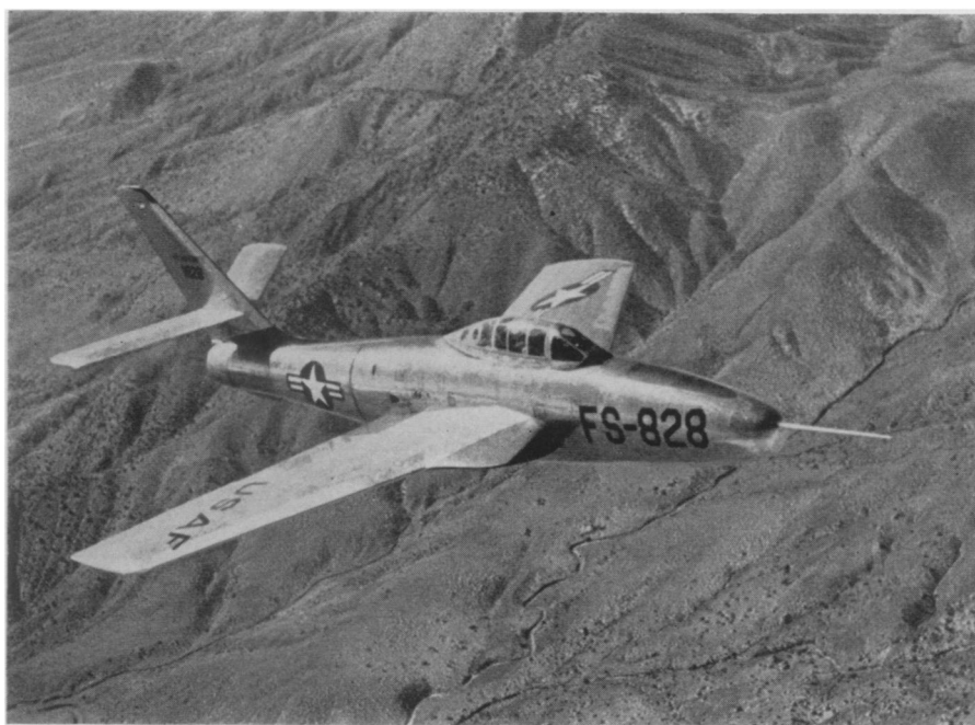
PHOTO RECONNAISSANCE PLANE —The RF-84F high-speed, high or low altitude, day or night photo reconnaissance plane, carries four .50 caliber machine guns for armament. Although performance details are under security wraps, it flies very much faster than the Thunderjet.
