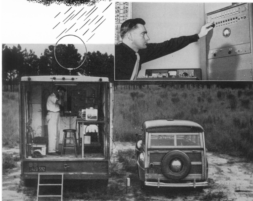
Thunder hunting equipment on location near Madison, Florida. Loop antenna on truck picks up static. The engineer in top picture is watching the indication of a circuit which registers how often the static exceeds a given level.
