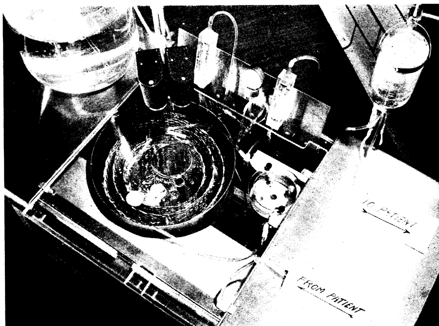
PLASTIC KIDNEY —This top view of the plastic kidney shows how the machine performs the same function as the human organ in cleansing impurities from the blood. The electric-eye safety device in the center automatically shuts the kidney off if trouble develops.
