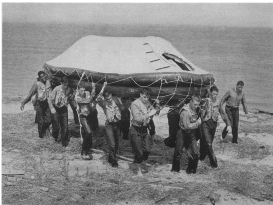
SPEEDILY SELF-INFLATED —In 30 seconds, this new life raft can inflate itself to give 70-degree protection for the 15 men, shown carrying the 230-pound boat.
