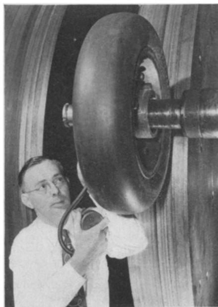
250-MILE-AN-HOUR TIRE—R. D. Van Arnamm here prepares a new tire to make simulated high-speed landings in the Firestone Tire and Rubber Company's laboratory at Akron, Ohio.
