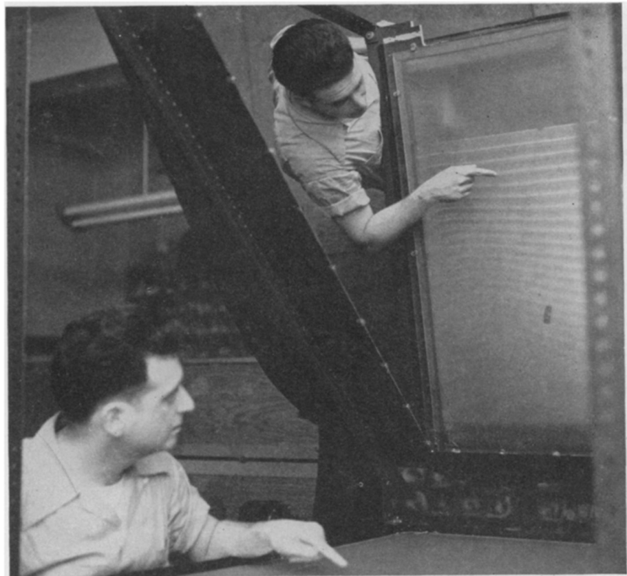
RIPPLE TANK —Oceanographer Wilbur Marks indicates the wave pattern created by a typical obstruction in the ripple tank, an instrument designed and constructed at New York University for the study of ocean surface waves. The effect of wave patterns on beach erosion is being investigated by the newly-formed department of meteorology and oceanography.
