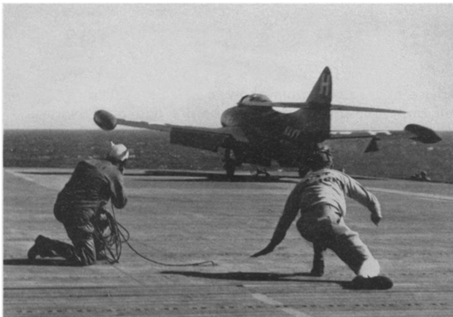
CATAPULT TAKE-OFF —A navy jet fighter taking off for Korea is here flung from the catapult of the USS Antietam as the catapult officer and the "talker" crouch to the flight deck to escape the blast of gases from the jet exhaust. The dropped flaps help to catch the wind.
