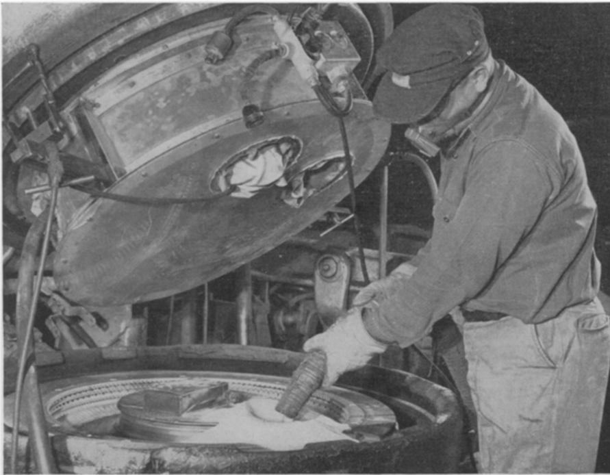
WALNUT SHELLS CLEAN —Walnut shells are now replacing sand or other materials likely to pit aluminum at The Firestone Tire and Rubber Company, Akron, Ohio. Using a vacuum tube, Chester Kanecke is drawing finely ground English walnut shells into the machine he uses to clean aluminum tire molds.
