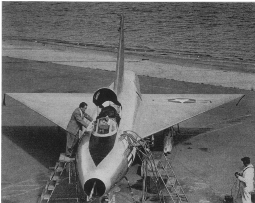
FUTURE PLANE'S SHAPE —The airplanes and rockets of the future, in the ranges beyond the speed of sound, will have the general configuration of this research craft, the Convair XF-92A delta wing research interceptor.
