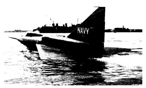
DELTA WING "SEA DART"—The Navy's revolutionary water based jet fighter, the XF2Y-1, has successfully passed its initial taxiing tests. The plane is the first jet fighter designed to land and take off from water as well as the first to use water skis to ease its water landings and take-offs. It is not expected to operate from the open sea like a carrier plane, but from protected waters.
