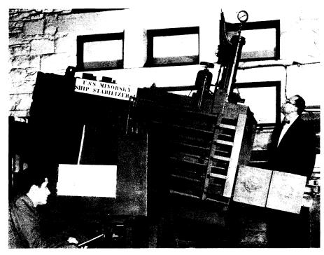
"HEAVY SEA" IN MINIATURE—The "U.S.S. Minorsky" rolls in a "hurricane," duplicating the real thing on a one-fifth scale. By turning a switch, engineers at Stanford University can activate a built-in automatic stabilizer and eliminate the rolling motion in seconds. Water tanks on each side, connected by a large pipe, rush water into whichever tank is on the rising side to give an even keel.
