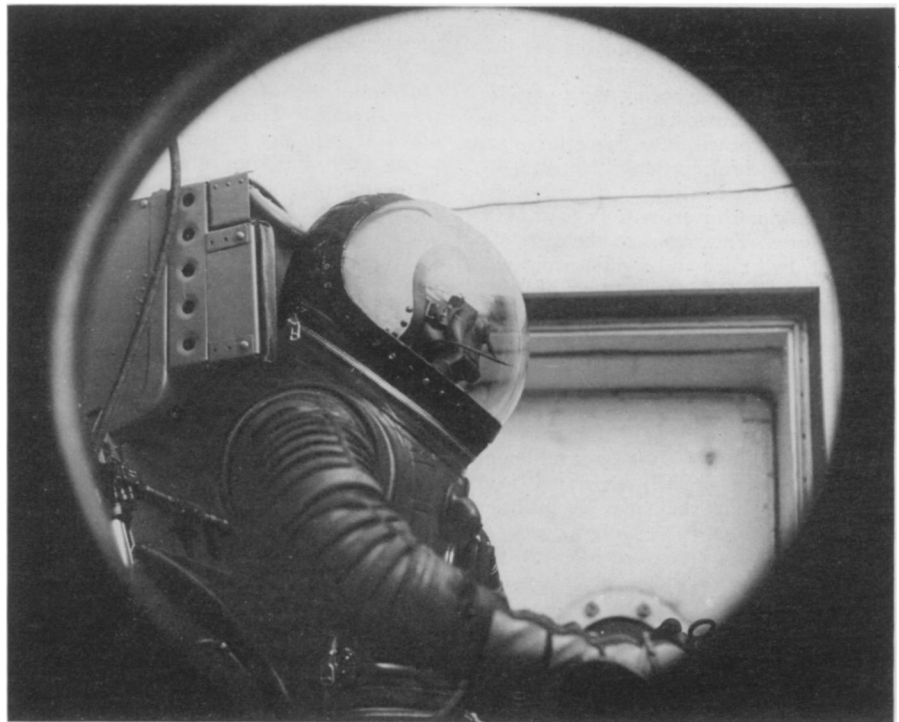
NAVY'S FLYING SUIT —Latest entry in the battle to keep humans alive in the frigid, nearly airless heights above 50,000 feet is this full pressure flying suit developed for the U. S. Navy.
