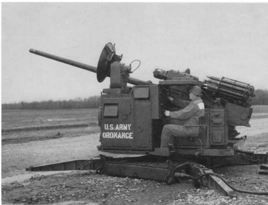
LARGEST AUTOMATIC GUN —The Skysweeper, a new 75 mm. anti-aircraft gun, has radar and computer mounted integrally with the weapon for quick and accurate spotting, tracking and interception of low-flying, high-speed enemy aircraft. Usable in all types of weather, the "artillery machine gun" can fire 45 twelve and one-half pound shells a minute. It was developed by Army Ordnance.
