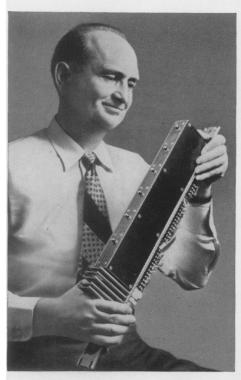
Laboratories engineer examines Transistor oscillator. It is used in Englewood, New Jersey, where 10,000 subscribers can personally dial distant cities. Transistors generate the signals which carry the dialed numbers to other towns and cities. Other uses are in prospect.
