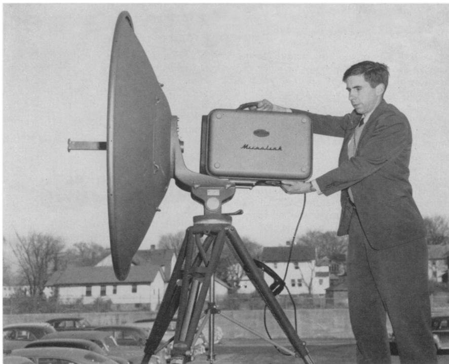
PORTABLE TRANSMITTER —Light enough to be picked up and moved about by one man is the small transmitter shown here. It was developed to speed sending of spot news from remote areas.
