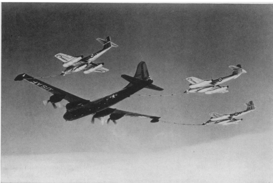
THREE AT A TIME —Multiple refueling of three Meteor jet fighters at the same time has been accomplished by a U. S. Air Force B-29, using the probe and drogue system manufactured by Flight Refuelling Ltd., Dorset, England.
