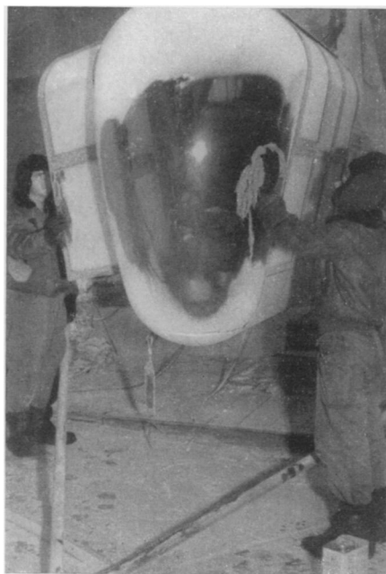
DEFROSTING HELICOPTER --Two U. S. Air Force technicians clean snow off the window panels of a helicopter after cold tests.
