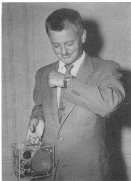
WRIST RADIO —While broadcasting into a wrist radio transmitter, James J. Sutherland of Sylvania Electric Products Inc. hears his own voice through the transistorized radio receiver he holds.
