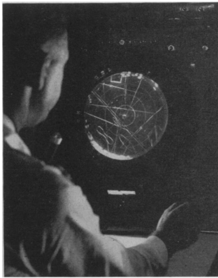
SCREEN OF NEW RADAR — The location of all moving aircraft within 30-to-60-mile radius can be spotted with this new radar.
