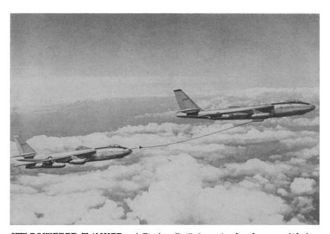
JET-POWERED TANKER—A Boeing B-47 Stratojet has been modified to make it an aerial refueling station, using a "probe and drogue" system. As shown in the photograph, the tanker airplane (right) trails a long hose, to the end of which is attached a funnel-like "drogue." The receiver airplane approaches the drogue, then engages the spear-like probe in its coupling mechanism, after which the fuel can be pumped.
