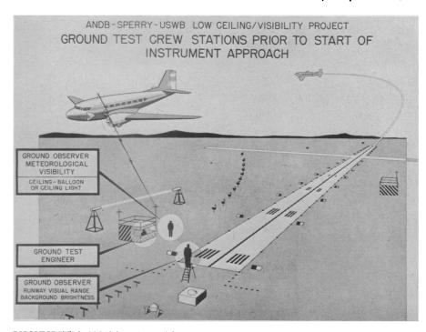
VISIBILITY INSTRUMENT LAYOUT—In addition to the instruments that measure visibility for landing aircraft, a weather observer climbs a stepladder to approximate the cockpit height at "touchdown." He records the number of "targets" he can see along, and to the left side, of the runway.
