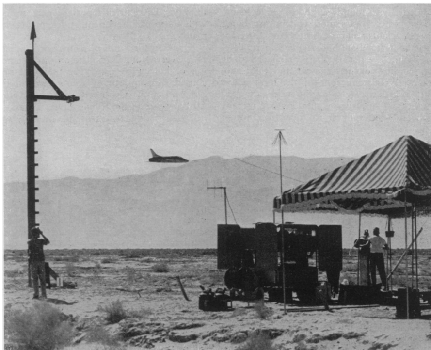
WORLD'S SPEED RECORD —Thundering to a new world's speed record is a North American Super Sabre, which on Oct. 29 averaged 754.98 miles per hour over a 15-kilometer course. The plane is powered by a Pratt and Whitney J-57 engine, which delivers 10,000 pounds of thrust.
