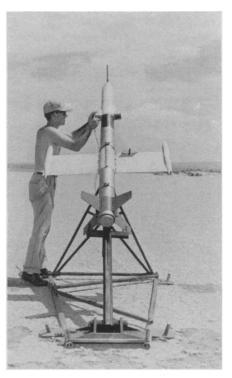
DESIGN TESTS—This rocket-driven device provides supersonic testing of scale models of wing designs for future aircraft. The model wing is mounted on a five-inch high-velocity combat rocket, and electronic instruments packed in the 74-inch rocket laboratory radio back to the ground reports on the wing's characteristics at speeds about twice supersonic.
