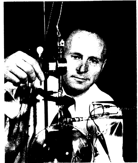
HIGH VACUUM PUMP —Dr. Anatole M. Gurewitsch adjusts a powerful magnet around a vacuum system using the new "ionic pump" developed by him and Dr. W. F. Westendorp of the General Electric Research Laboratory, Schenectady, N. Y. (See SNL, March 27, p. 200.)
