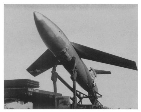
LAUNCHING POSITION—This is how the U.S. Air Force's B-61 Martin Matador, powered by a turbojet engine, looks when ready for launching. The first squadron equipped with the pilotless bombers is now in West Germany after training at Cocoa, Fla. It is the first overseas deployment of any unit using a pilotless, radar-controlled aerial weapon. The B-61 is platform-launched with the assistance of a rocket bottle that falls off when its thrust is expended.
