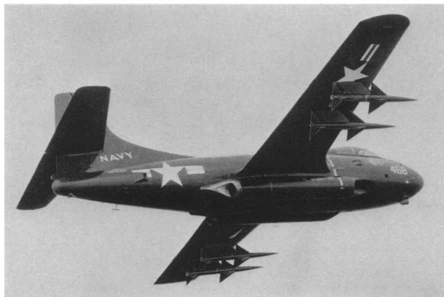
AIR-TO-AIR MISSILES —This is the first photograph of the Sperry Sparrows, air-to-air guided missiles that hurtle toward their targets at supersonic speeds. They are poised on wing racks of the Navy's twin-jet night fighter, the Douglas F3D Skynight.
