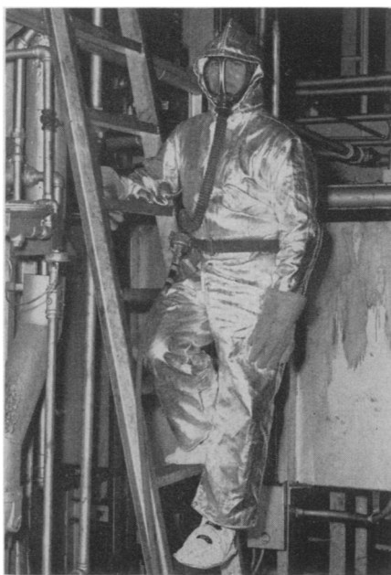
HIGH-TEMPERATURE SUIT— This man is wearing an aluminum-coated suit that reflects 90% of the heat encountered between two tunnels of a huge gas furnace at the Belleville, N. J., plant of Walter Kidde and Company. The air-cooled garb permits him to work 45 minutes in temperatures of 400° Fahrenheit.
