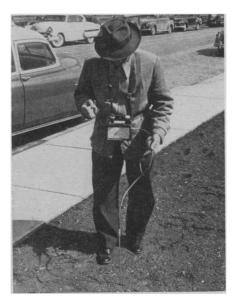
underground pipes and analyze gas concentrations both within and above or below explosive limits. The detector, which operates on flashlight batteries, is small and lightweight, as shown in the photograph.
