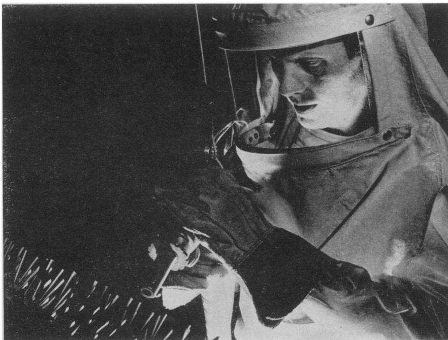
"BLAST OFF" —Instead of the deadly ray of science fiction stories, this operator uses rice hulls and ground walnut shells to blast off surface dirt on General Electric J-47 jet engines returned for overhaul.
