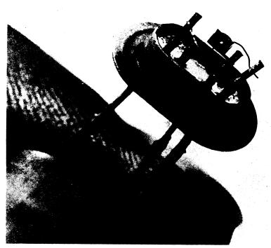
TRANSISTOR FOR AMPLIFICATION—This new ultra-high-frequency transistor can increase an original electrical impulse a thousand-fold when used as an amplifier. To date, frequencies as high as 440,000,000 cycles per second have been generated, about four times that of any comparable transistor. Scientists at Bell Telephone Laboratories foresee use of the device in the family TV set and portable radio sets.
